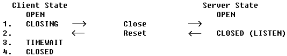
Fig. 6-3. The procedure of connection being closed by client.
