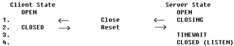
Fig. 6-4. The procedure of server holding TIMEWAIT state.
