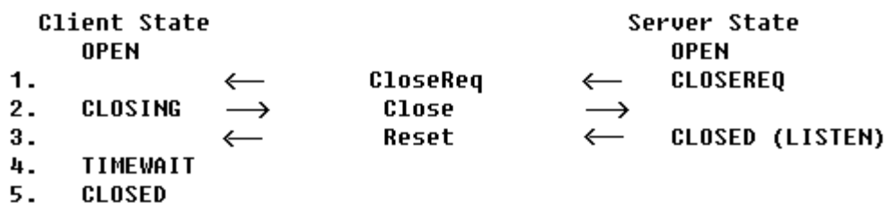
Fig. 6-2. The procedure of normal connection termination.
