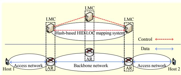
Fig. 5. Network model for HID-LOC mapping control.
