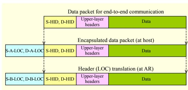
Fig. 4. Data packet encapsulation and LOC translation.
