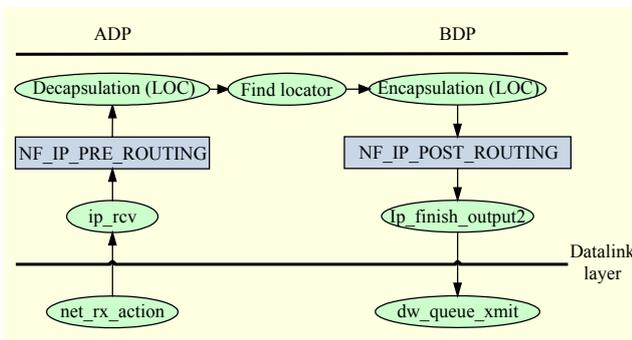
Fig. 11. Netfilter modules used for AR implementation.
