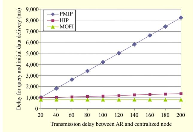
Fig. 19. Delays for LOC query and initial packet delivery by transmission delay between AR and central agent.
