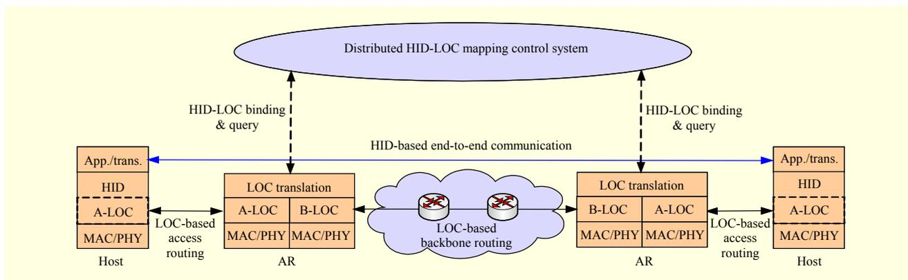
Fig. 3. Query-first data delivery with mapping system.
