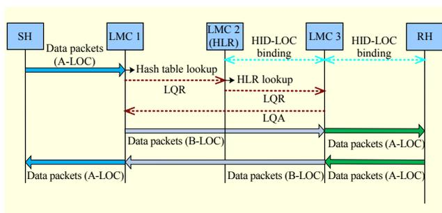
Fig. 7. LOC query operation for data delivery.
